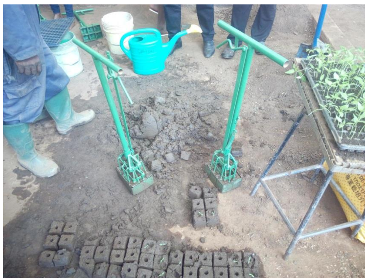
Fig 2: Equipment used to make soil blocks.
