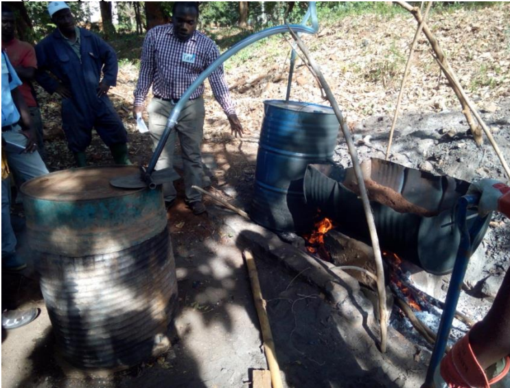
Fig 3: Soil sterilization using the drum and steam method.
